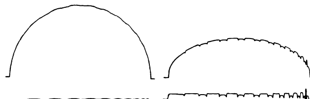
FIG. 1. Effect of convolution on ellipses. The function g (Upper left) is a large ellipse with small elliptical bumps (Lower left); 0.5g + 0.5k*g and k*g are shown (Right).
